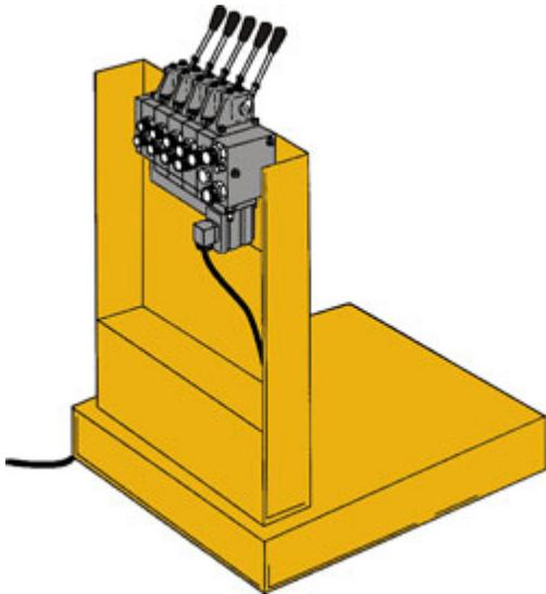
This system can have the main control valve mounted in any convenient position (remote from rockbreaker). Available stand for the valve, for mounting in an existing operator cab, or on or near the operator platform. An electric foot switch fires the breaker. Hose length up to 30 ft (max recommended) Remote manual hose kits are available..
