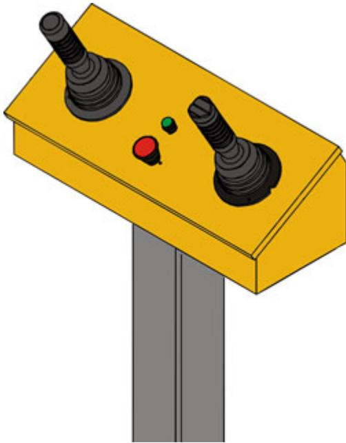
Two dual axis joystick controls with a right-hand thumb switch for breaker fire. Controllers are mounted on a compact control stand making it easy to locate in a crusher control room. An indicator "on" light and a joystick power shutdown button (shutting down power to control valve only) are located on the stand between the controllers.
