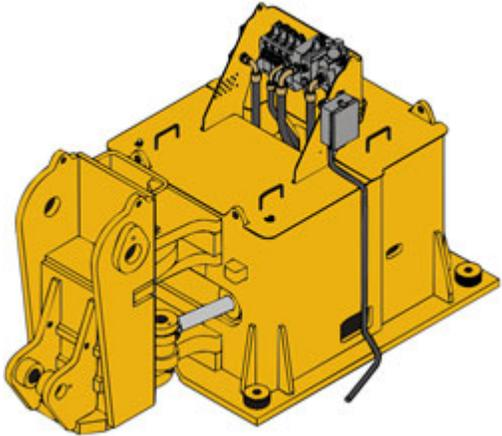
Main controls are mounted on the pedestal. Uses a spring return to neutral hydraulic control valve, manually operated with four levers, providing independent control of all boom functions. The breaker fire control uses an electric foot switch providing positive (instant) control of the breaker. This is used in conjunction with the selected joystick.
